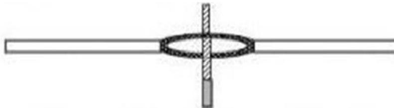
C) Wrap the connected wire on both sides of the connection to form a knot and pull connection tight.
