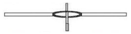
c) Wrap the connected wire on both sides of the connection to form a knot and pull the connection tight.
